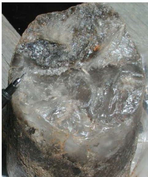
Figure 14 – Core of Coarsely Crystalline Halite from Area. (From McKillop, et al. , 2007)
