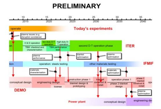
Such a plan shows why it will be very difficult to commission the first commercial-sized tokamak before 2050. However it could be that sufficient information is gained on the step beyond ITER (DEMO), through its staged operation, and it is sufficiently prototypical of the series production of power plants, that it will be possible to be more confident at an earlier stage concerning the <u>economic viability</u> of the first series of power plants produced.
