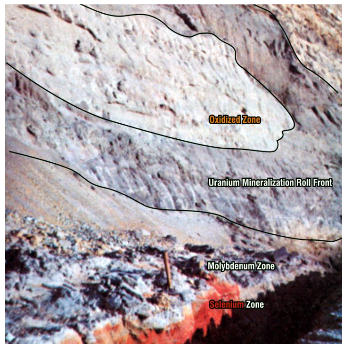
Figure 1 - Typical Uranium Roll Front in Wall of Open-Cut Mine in South Texas from the 1970s (After Dickinson and Duval, 1977).
