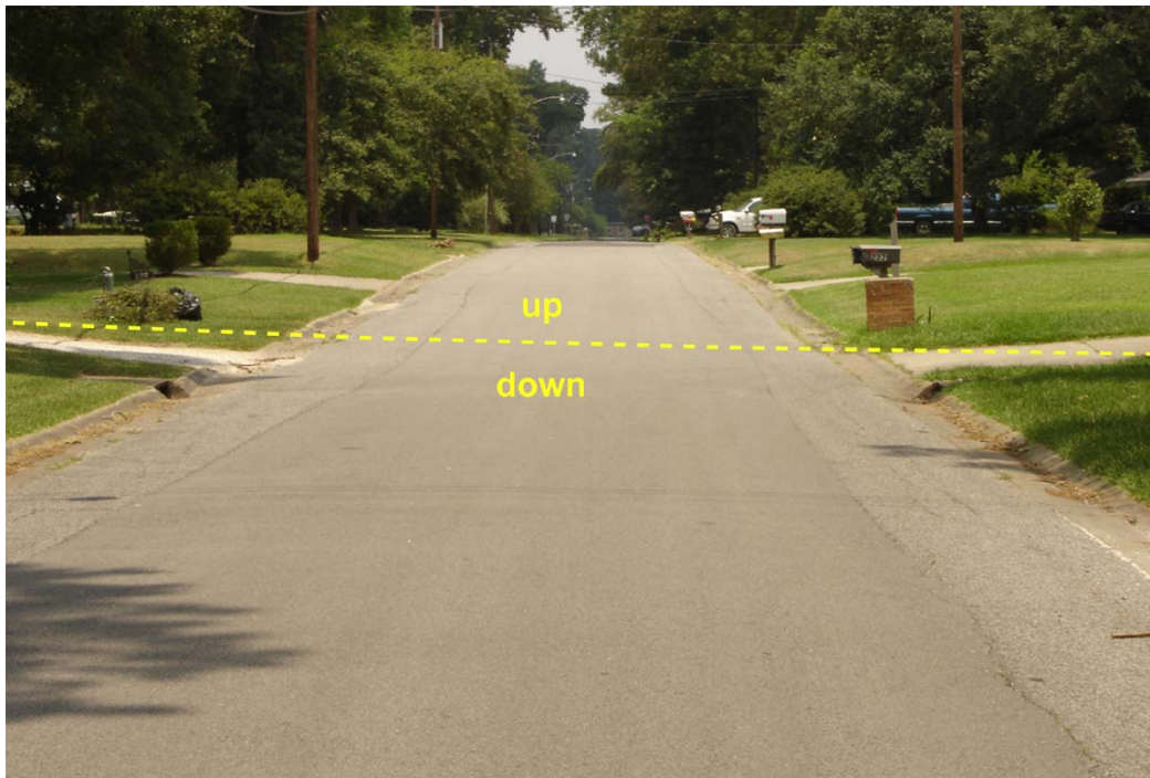
Figure C.4. Photo of the Sulphur fault-related step near Westlake. The dashed line represents the approximate location of the fault trace.
