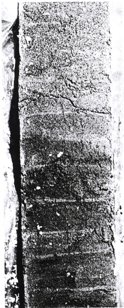
FIGURE 2. Redox Interface. The induced oxidation of chemical leaching. Dark area of core is ore material; lighter area above has been leached to remove ore.
