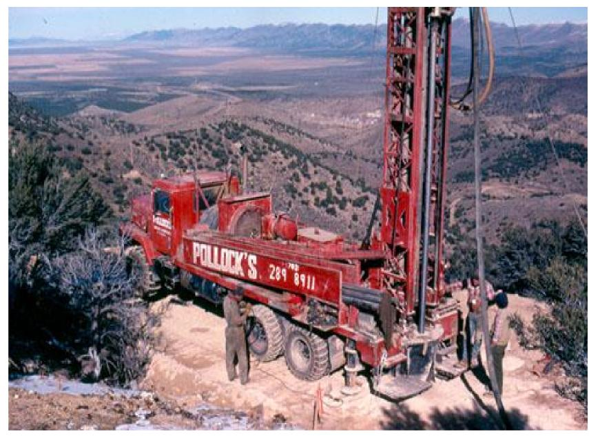
Reverse-Circulation Rotary Drilling
