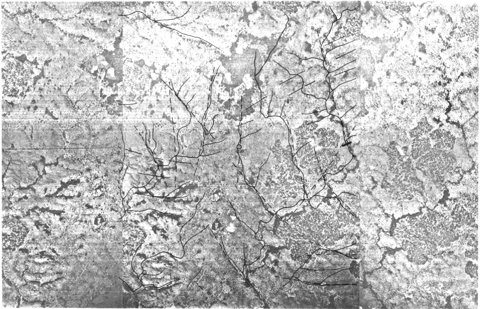
Image 6. Stereo pair showing a biotite-hornblende gneiss in Tanzania. The strike directions of the gneissic bands can be recognized even when covered with bush. The drainage reflects partly the fractures but also the strike directions of gneiss bands (see overlay). Approximate scale 1:40,000.
