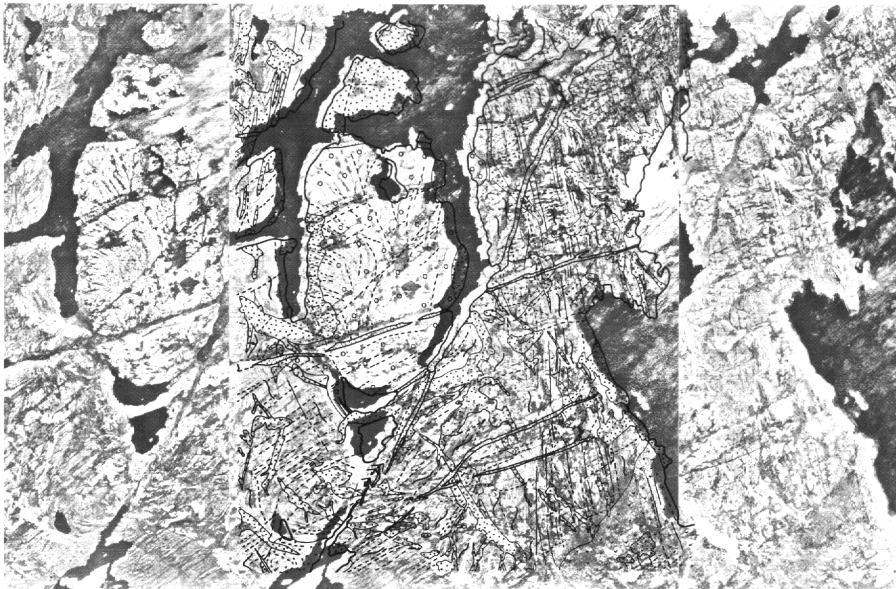
Image 4. Stereo triplet showing intrusive body of granite (light-tone) in highly metamorphic folded basement rocks (medium tone). Most fracture lines have been intruded by dikes. The aplitic and pegmatite dikes show light phototone and relatively strong relief; the basic show darker tone (see overlay).
